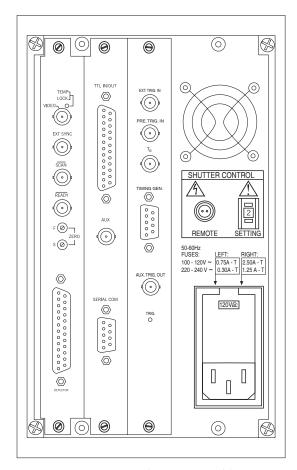
Figure 31. ST-133 with Programmable Timing Generator and PCI (TAXI) Interface Control Module
